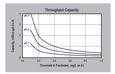
**CAPACITY** — The graph above is based on waters with TDS less than 500 ppm and is for chromate alone, exclusive of other anions. Capacity shown is for the working bed in a worker polisher configuration. No engineering downgrade has been applied. Suggested System Configuration
